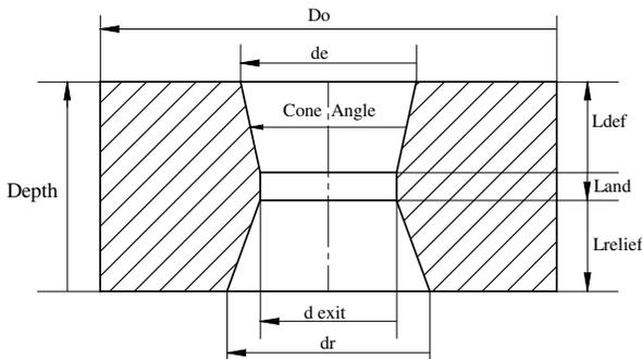
Fig 1: Conventional Die with all parameters
