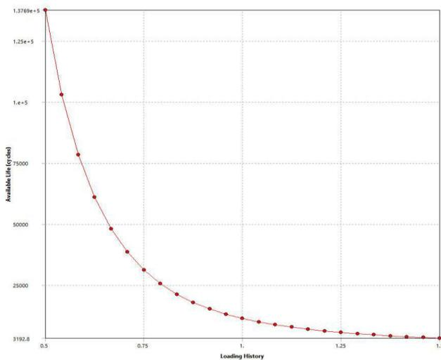
Fig 6. Life cycle of die with respect Load factor
