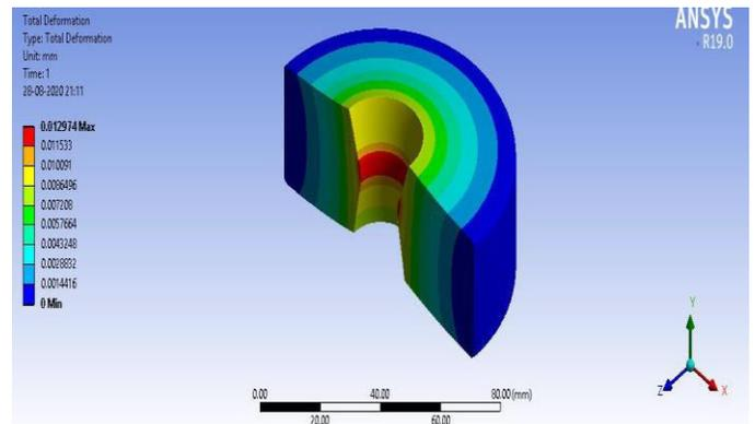
Fig 2. Total Deformation for 90mm Diameter Die.
