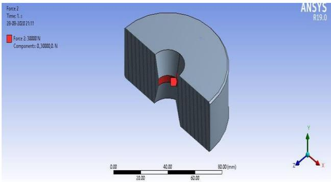
Fig 4. 30KN force applied to the die at the land position.
