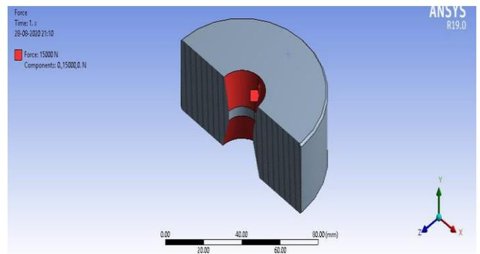
Fig 3. The Force 15000N applied to 90mm Die the at upward position
